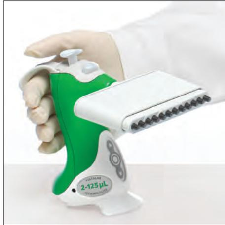
The Ovation pipette has been designed to allow the body of the pipette to fill your palm. Rotate the adjustable hook to rest comfortably on your forefinger. The texture of the unit's back helps reinforce correct hand positioning.
