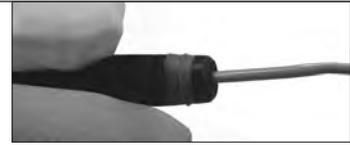
2. Pick up a new nozzle filter with tweezers and place it into the wide (threaded) end of the nozzle.
