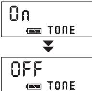
1. Simultaneously press and hold the  $\wedge$   $\vee$  buttons until **TONE** appears on the display.
