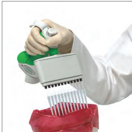
The Ovation multichannel pipette stores energy captured during the acquisition of tips, and uses it to discard tips when the tip eject button is pressed. Point pipette tips into a suitable waste container and gently press the button. The ejector slide is activated, discarding all tips simultaneously.
