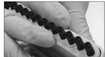
2. Remove the affected nozzle(s) by placing the rubber tubing provided onto nozzle, and unscrew it in a counterclockwise direction. If it is suspected that the air tube has been contaminated, gently wipe the end of the air tube with a tissue, then dry it off. To remove a nozzle(s) on 0.5–20 L models, use the nozzle removal tool supplied with Replacement Nozzles or the Nozzle Reconditioning Kit.
