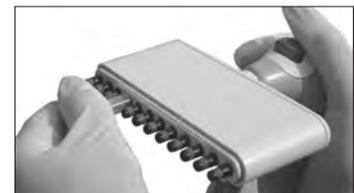
3. Place rubber tubing onto a new nozzle (or nozzle where filter has been replaced), and screw the nozzle onto the pipette in a clockwise direction. Firmly tighten and remove tubing from nozzle.
