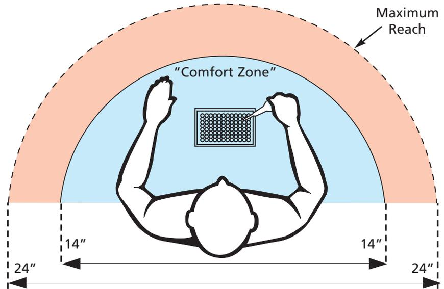
Ergonomics experts recommend establishing a "comfort zone" of movement for the task of pipetting. Position your body within 9" of the counter surface, and keep the items needed within easy reach. Ideally this should be 14" or less, and should not exceed 24" of occasional reaching. Wrist rotation should not exceed 90° from the work surface, and arm/hand elevations should not exceed 12".
