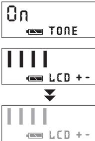
1. Simultaneously press and hold the  $\wedge$   $\vee$  buttons until **TONE** appears on the display.
