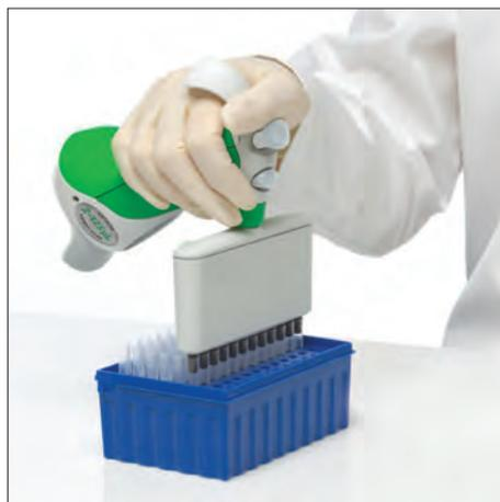
While maintaining a flat wrist-hand posture, insert the Ovation pipette nozzles into a row of tips. If desired, place other hand on the textured surface (top) of the tip head and press down until you hear or feel a "click" and the indicator line on the tip head is hidden. This indicates that the tips are properly seated and ready for use.
