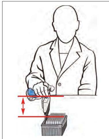
*Arm elevation remains low, minimizing stress to elbow, shoulder and neck*
