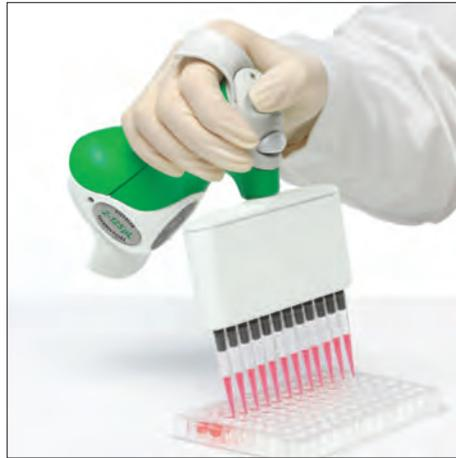
Smooth gliding movements of the upper extremities with proper posture and minimal stress is the key to ergonomically correct pipetting. Maintain a low forearm elevation and neutral wrist posture throughout the pipetting cycle. Immerse pipette tips to an appropriate depth (1mm for 0.5–20 $\mu$ L, 2 to 3mm for 2 $\mu$ L–125 $\mu$ L & 5–250 $\mu$ L, and 2 to 4mm for 25–850 $\mu$ L). Press & release the pipetting trigger to aspirate sample. Press pipetting trigger again to dispense or mix sample.
